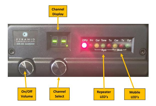
On/Off/Volume: Disabled. These functions are controlled via the mobile radio interface.
