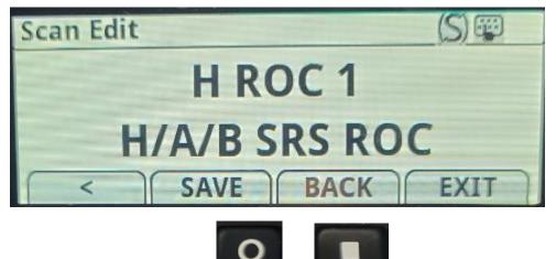
While in Scan Edit mode, pressing the **second** or **second** button will toggle through the channels currently assigned to the scan list. Save. The (S) in the upper right display corner designates the channel has been added to the scan list.
